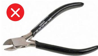
Electrician's Side Cutters NOT RECOMMENDED
