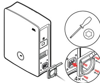
This completes the replacement of the charging socket flap. If necessary, repeat the procedure for the wallbox's second charging socket.
