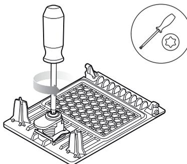
5 Remove the bracket for the lock with the slotted screwdriver.
