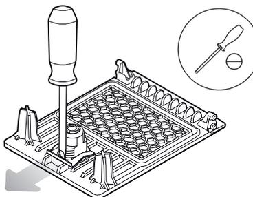
6 Push the lock downwards out of the opening in the RCCB flap.
