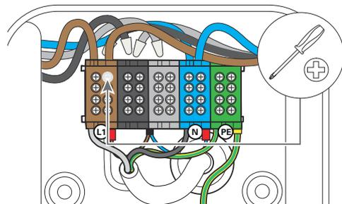
The charge points of the Wallbox eM4 Twin are now electrically set up for single-phase operation. In addition to the electrical conversion, however, you must also set up the wallbox for 1-phase operation via the **ABL Configuration App**. To do this, please refer to the sections starting on page 40.
