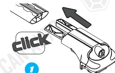
**EN** Insert the lockable feet into each end of the aluminium bar. Ensure the foot is fully inserted until you hear a "click".
