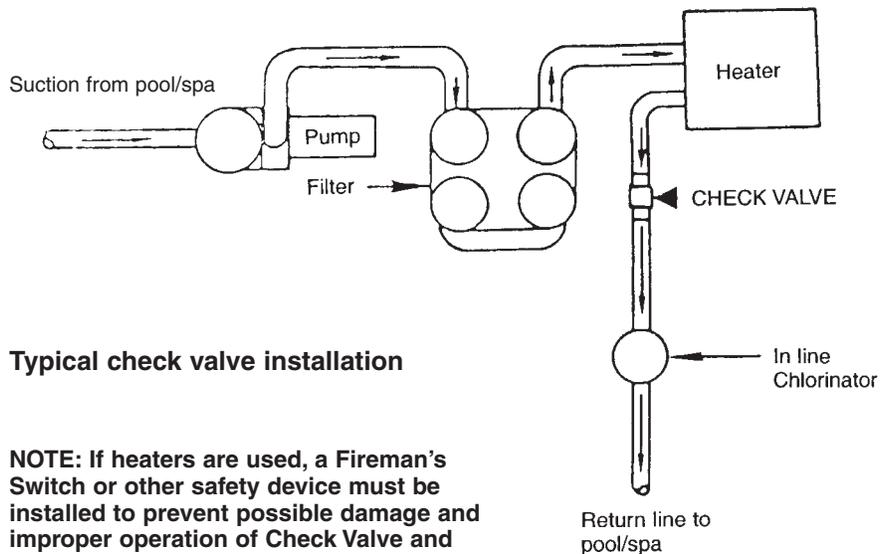
**Typical check valve installation**
