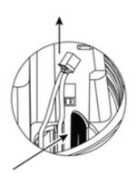
5. Take the new battery and place it at the bottom of the cavity until it is secure. Then, plug in the connector.
