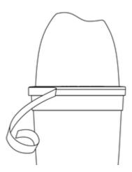
3. Remove the adhesive tape and unscrew the upper part of the device. This is a left-hand thread. Unscrew it in a clockwise direction. Remove the seal and discard it.
