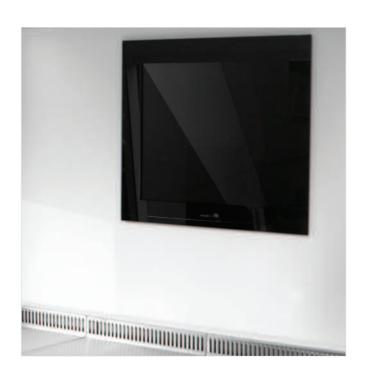
Built-in LAF-LCD screen mounted on the rear wall or alternatively magnetically attached, for easy removal or positioning to suit the operator's convenience and comfort.
