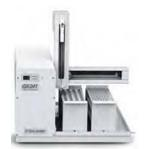
The GX-241 Liquid Handler offers a two-rack platform for large or small volume injection and automatic fraction collection using tubes, vials, or microplates. Its small footprint makes it an ideal choice for labs where bench space is limited.
