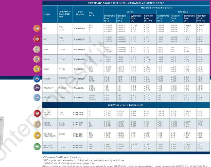
Gilson maximum permissible errors are guaranteed only when PIPETMAN® pipettes are used with the recommended PIPETMAN® DIAMOND Tips
