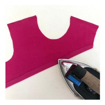
Press the lower edge of the top front to the back side following seam allowance line at 1,5 cm.
