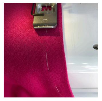
Sew basted seams of the top and bottom fronts using coverstitch machine. Try to position the stitching in such a way that the basting hand stitch is in the middle between coverlock needles.
