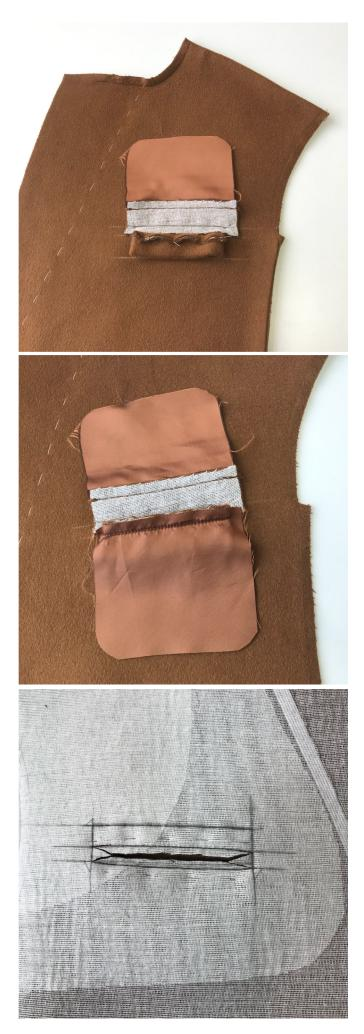
Fold the welt seam allowance toward the welt and pin. Place the pocket facing on top of the front piece, right sides together, match the seam allowances of the facing on the front and the pocket bag, stitch the pocket facing with the pocket bag. The stitching line of the facing must be 2mm shorter than that of the welt on each side. This will ensure that the finished welt will cover the facing seam completely.
