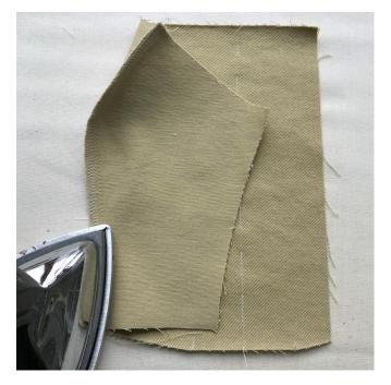
Finish the seam allowances on the overlocker. Overlock with the side front bodice facing up. Press the seams flat.
