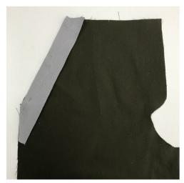
Place the pocket facing piece right sides together with the front leg pocket opening. Pin, baste, and stitch on the machine. Backstitch at the beginning and end.
