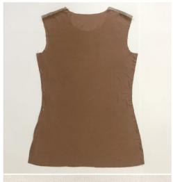
Place the front and back pieces right sides together. Align the shoulder and side seams, pin, baste, and overlock with the back piece facing up. Stitch width is 7mm, so trim off 3mm while serging.
