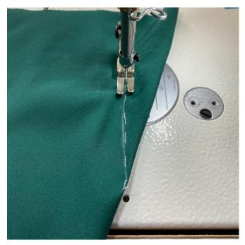
Machine-stitch the darts. Backstitch at the raw edge and leave long thread tails at the dart point.
