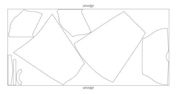
Interfacing, 140 cm (55") wide, cut on a single layer in one direction, for all sizes in all heights
