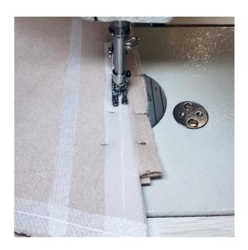
Machine-stitch the dart, backstitching at the beginning and end. Start stitching on the second strip, 1 cm (3/8") below the dart point, and then continue stitching along the entire length of the dart.
