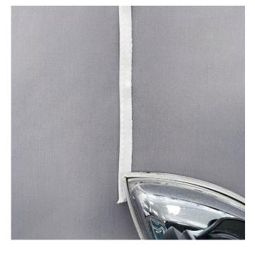
Press and steam the piping in order to prevent its shrinkage in the finished garment.
