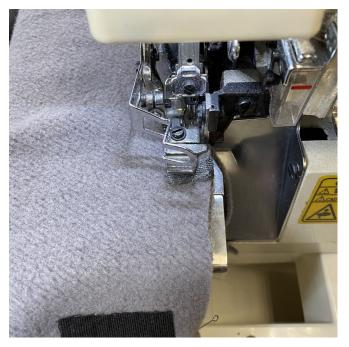
Stitch the side seams on the overlocker, keeping the front piece facing up.
