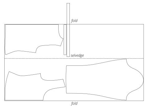
Attention! The back neck binding piece is cut once. The front neck binding piece is cut once on a single layer out of the leftover fabric.
