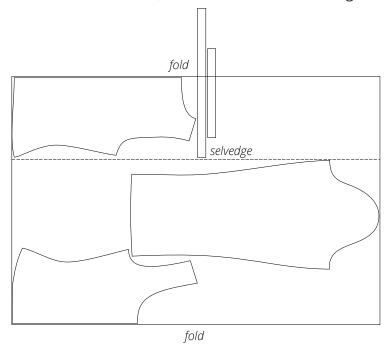
**Attention!** The back neck binding and front neck binding pieces are each cut once on a single layer from the leftover fabric.
