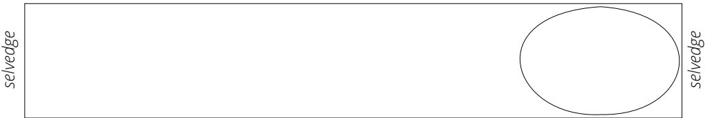
Stiffener (2 mm EVA), 140 cm (55") wide, cut on a single layer
