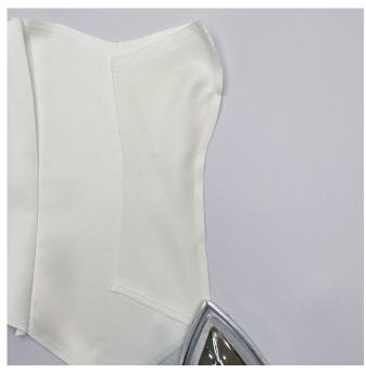
Stitch on the sewing machine, backstitching at the beginning and end of the seam.
