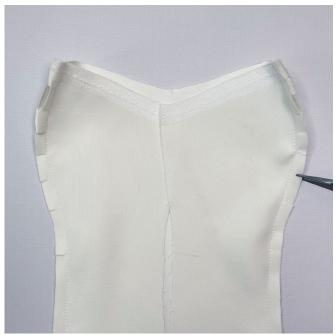
Clip into the curved sections of the princess seam allowances, stopping 2 mm short of the seam.
