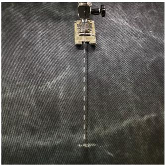
Using a 3.5 mm stitch length and topstitching thread, topstitch the darts from the right side at 1–2 mm from the seam to secure the dart seam allowances.
