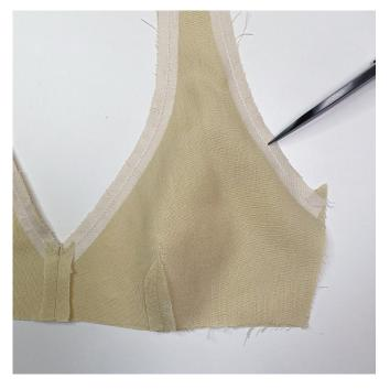
Clip into the curved areas of the armscye and neckline seam allowances every 1–1.5 cm (3/8–5/8"), stopping 2 mm short of the seam.
