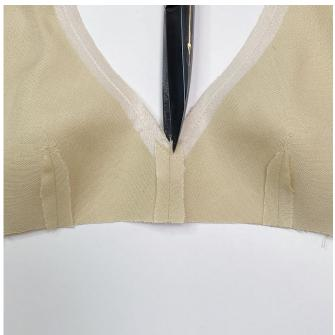
Clip into the corner, stopping 2 mm short of the stitching line.
