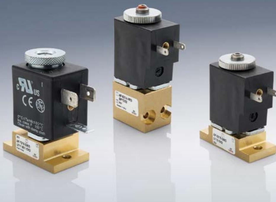
Series AP directly operated 2/2-way proportional solenoid valves, NC, with nominal diameters range from 0.8 to 2.4 mm, can be used where an open loop flow control is required, with gas mixtures, to control free flows or blows, or emptying chambers using vacuum.
