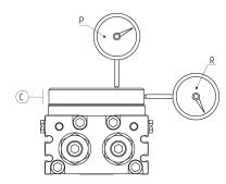
P = Parallelism of the rotary table 0,1mm R = Roundness of the rotary table 0,1mm C = Cylindricity of the rotary table 0,1mm
