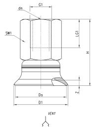
Tolerances for elastomer parts according to M3 - DIN 7715
